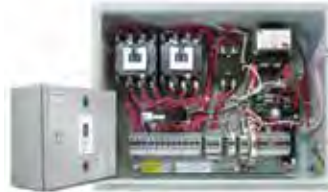
PYROBOX 3C Power management electrical box 2 x 3 poles 50A / 600V contactors with ground fault
